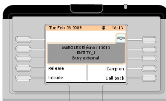
Figure 2.12: Telephone Area Example (the Called Set is in Conversation with External Party)
