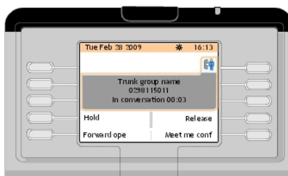
Figure 3.1: Telephone Area Example (External Call in Conversation)
