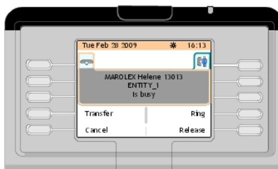
Figure 2.46: Telephone Area Example (Internal Busy Set Number Dialed)
