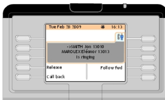
Figure 2.19: Telephone Area Example (the Called Set 13013 is in Forward on No Answer)
