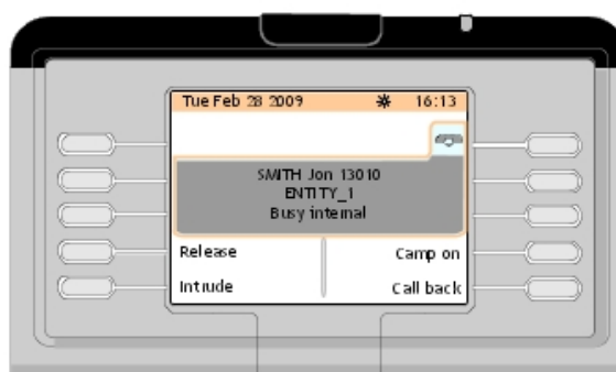
Figure 2.22: Telephone Area Example (Forwarded on Busy Set 13010 overrides the Forwarding Destination Set )
