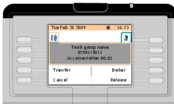
Figure 2.44: Telephone Area Example (External Second Party is in Conversation, Internal First Party is On Hold)
