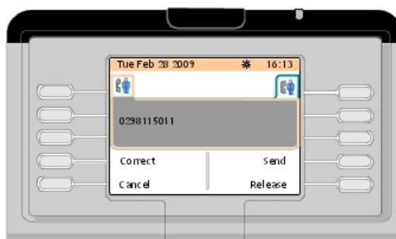
Figure 2.43: Telephone Area Example (All Digits of the External Number Dialed)
