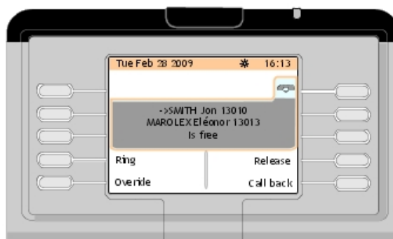
Figure 2.17: Telephone Area Example (the Called Set 13013 is in Immediate Forwarding)
