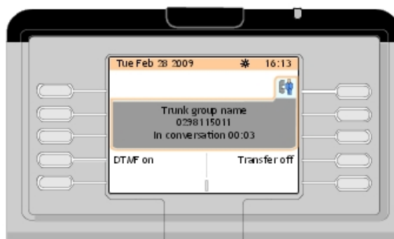
Figure 3.10: Telephone Area Example (External Call in Conversation)
