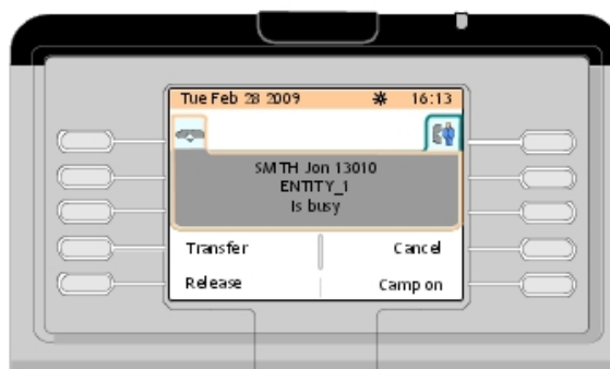
Figure 2.47: Telephone Area Example (Internal Busy Set Number Dialed)
