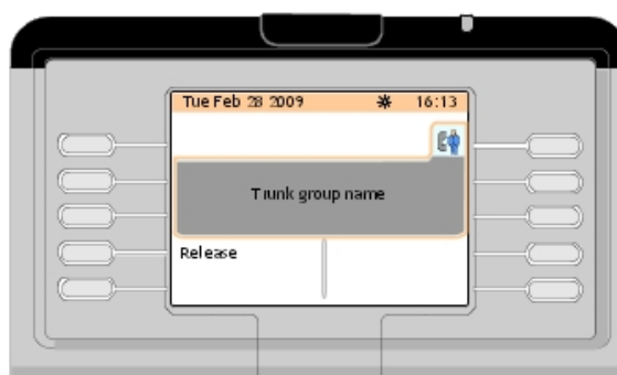
Figure 2.23: Telephone Area Example (External Access Prefix Dialed)
