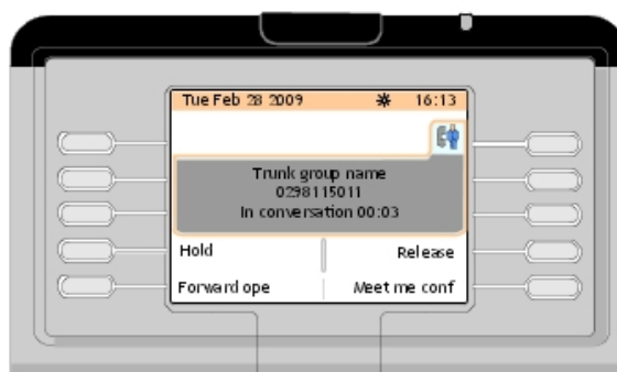
Figure 3.5: Telephone Area Example (External Call in Conversation)
