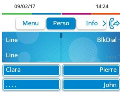
User interface with virtual add-on. 4 programmable softkeys are displayed and can be used as a smart add-on module.
